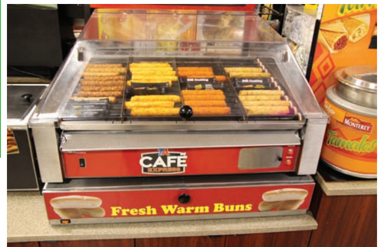
The most energy efficient grills today seal the ends of the hollow rollers, preventing the heated air from escaping, allowing the use of significantly lower wattage heating elements, saving up to 20% in energy costs.
